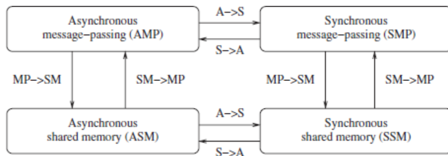
Figure: Emulations among the principal system classes in a failure free system.
